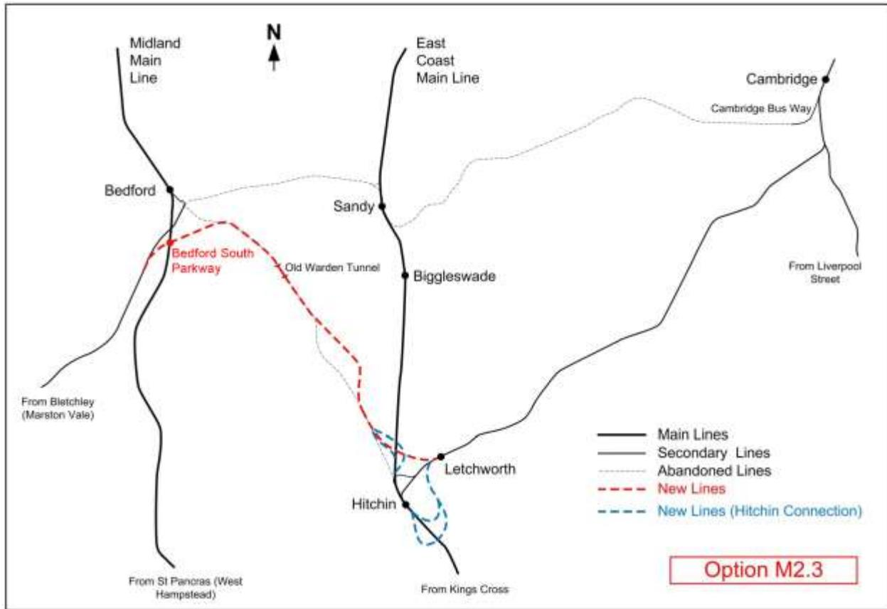
Figure 1.1 – M2-3 Alignment Options (Phase 2a Report Alignment)
