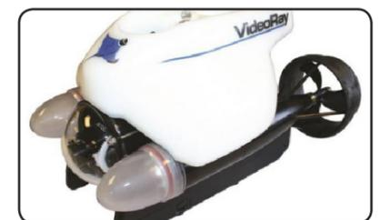
fig. 5 - Submersible remote camera
